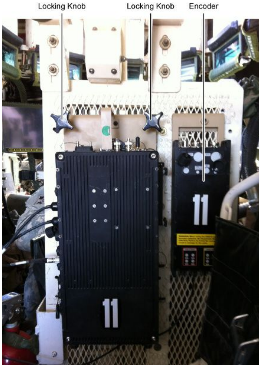
Figure 4-54. CMUR Front View
