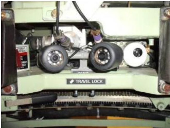
Figure 4-41. Crew Cameras and M2/M3 Camera Bracket Installed
