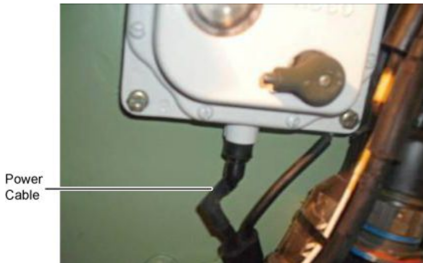
Figure 4-62. Dome Light Power Cable
