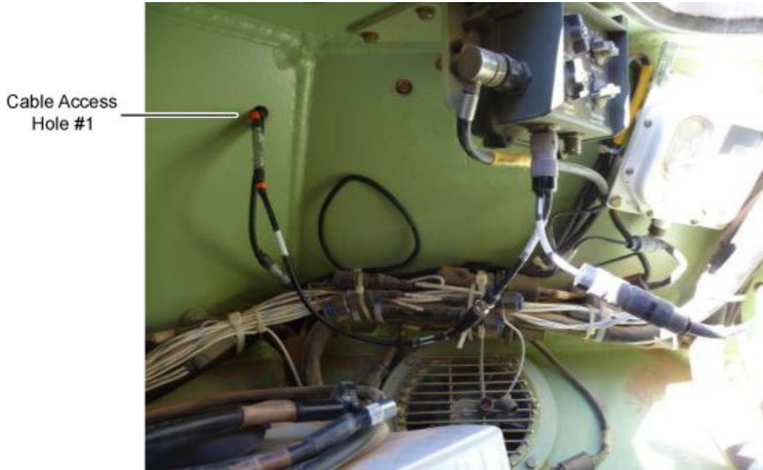
Figure 4-29. Cable Access Holes Behind Gunner's Position (Inside View)
