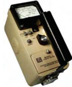
Figure 2. General Purpose Survey Meter
